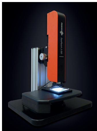
The LED ringlight provides incidental uniform white illumination to the entire membrane filter patch.
